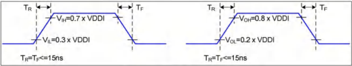
Rising and Falling Timing for I/O Signal
