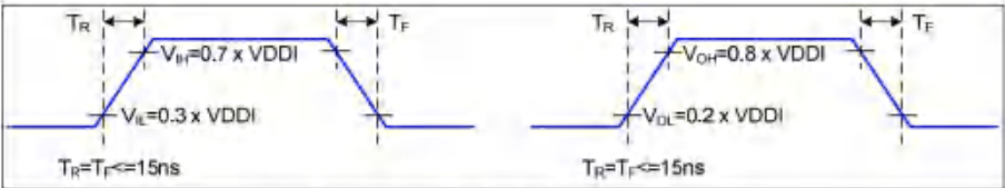
Figure 2 Rising and Falling Timing for I/O Signal
